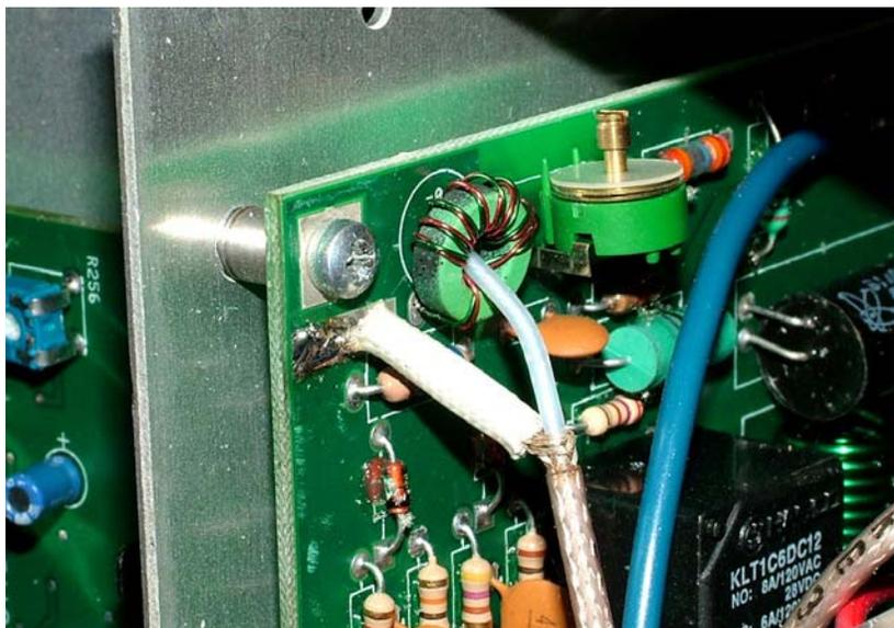
Step 9: Route the other coax cable (RF OUT) from the JT-11 to the SO-239 connector on the back of the radio. The RF OUT cable is attached to the back of the JT-11 board to a solder pad labeled "Antenna". Solder the cable to the connector; the coax center conductor goes to the center pin of the connector. Again, use the insulating sleeve from Step 7 to insulate the shield before soldering it to the ground lug on the connector.
