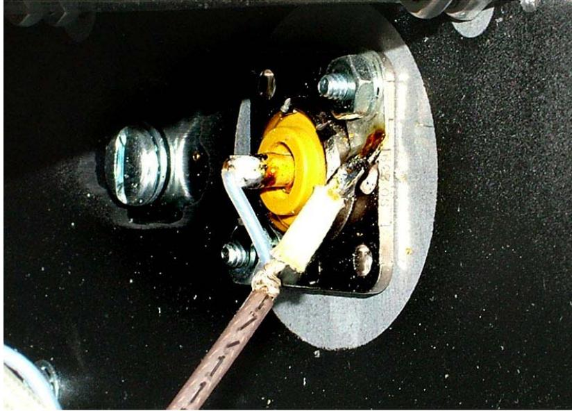
Step 10: Reattach the FILTER board to the chassis using the screws you removed in Step 6. Do not overtighten.
