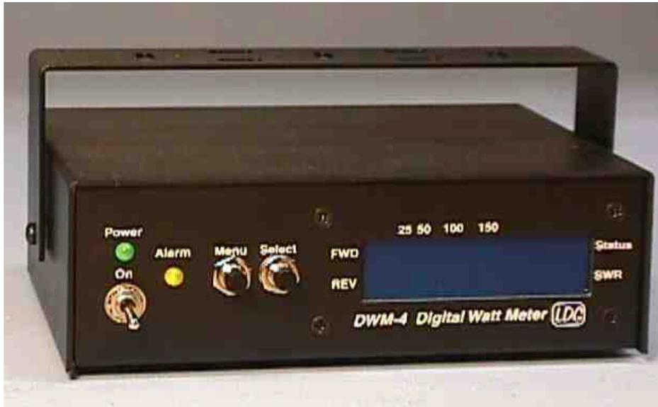
**Introduction:** The DWM-4 is a four channel, microprocessor controlled RF wattmeter. It consists of two main parts, the display unit and the remote sensor. The display unit has a 2 by 16 backlit LCD module that provides the user with information about the RF that is being sampled by the remote sensor. The user can simultaneously view forward power, reverse power and swr on the same display for instant analysis of the antenna system.
