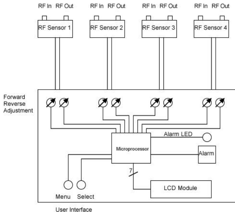
**Operation:** Turning the display unit on will show the model and software version of the DWM-4. The power LED is software controlled, so it will only come on if the software is running properly. You may have to adjust the contrast pot (R25) fully counter-clockwise to properly view the LCD module information. After the display comes on, adjust R25 for best view.
