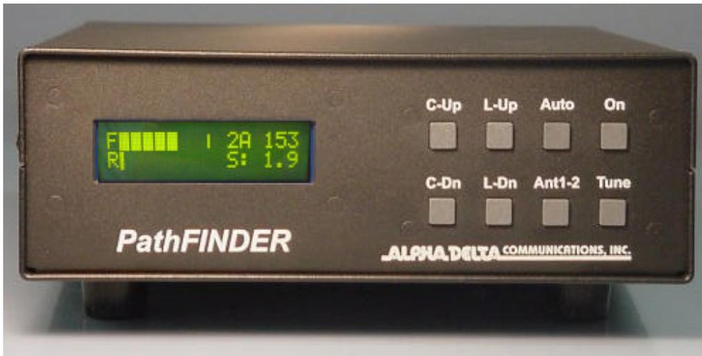
**Operation:** Once the PathFINDER is connected and the display is on, the user can operate the front panel controls and observe the changes in the display. There are eight front panel momentary push buttons. Some buttons provide more than one feature and some buttons are used in combination to provide additional features.
