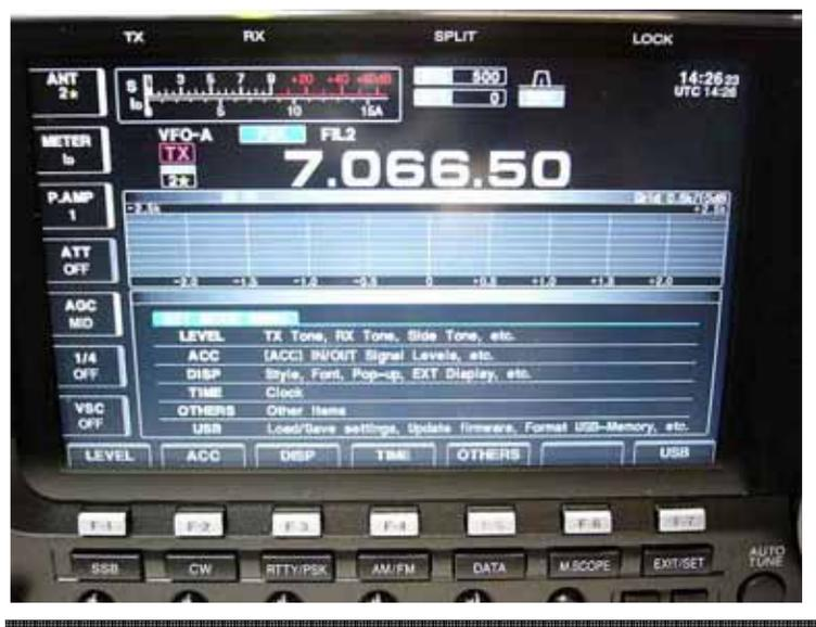
Next, press the **F2 (ACC)** soft button. Using the **F1 (down)** and **F2 (up)** soft buttons, scroll down until the **External Meter Output** item is selected. Rotate the main dial knob until **V<sub>D</sub>** is selected. This displays the output drive transistor voltage, which should be constant at 48 volts.
