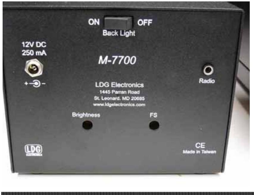
The DC Coax jack accepts a 2.5 x 5.5mm coaxial DC power cable, 12V, 250mA, center positive. External power is only required if use of the internal backlight is desired. The meter functions correctly otherwise without it.
