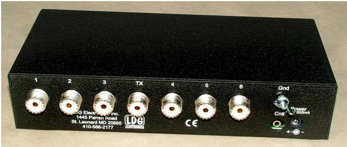
The 2.5 x 5.5 mm jack coaxial DC power connector is on the right. The ground connection is via the wingnut. The control cable input is a 1/8" stereo jack; the control cable is included with the DTS-6R remote.
