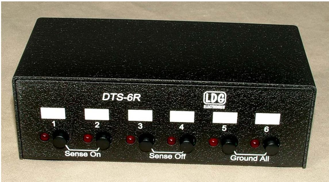
The DTS-6R remote is smaller than the DTS-6, but has the same six switches and six LED lights on the front. On the back, it has the same power, and control jacks, and a radio sense connector, but of course no coax connectors.
