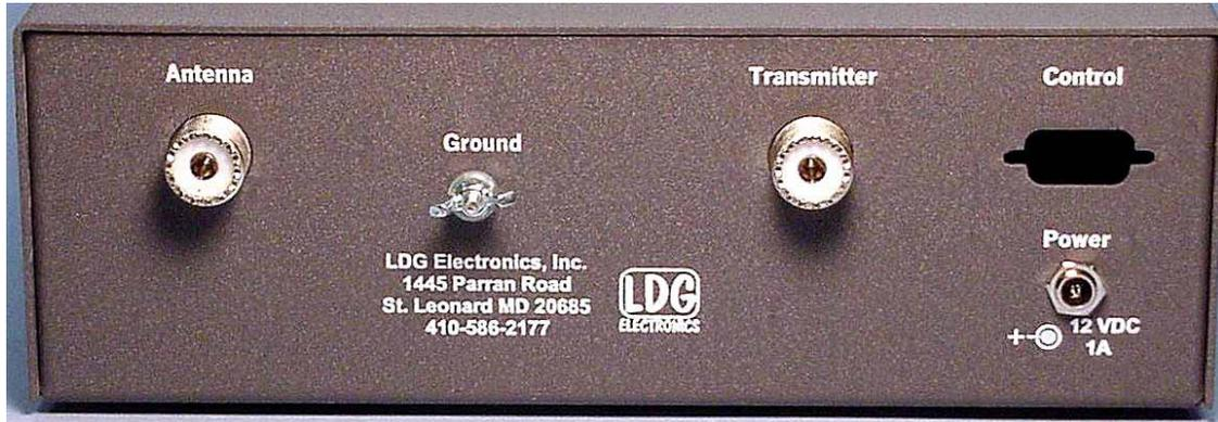
“What’s the deal with the hole?” Sharp-eyed users will note an empty cutout labeled “Control” on the back panel. Future versions of the AT-1000 may feature remote control and monitoring via a DB-9 connector in this position. This feature may also be offered as an upgrade for present users, but is not available at this time. In this version, the cutout serves no function. Never insert anything into this cutout, especially when transmitting.
